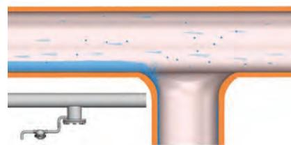
**FIGURE 3.** Steam contains condensate, both entrained in vapor, and disentrained flowing along the bottom of the pipe as a liquid stream. Only already disentrained condensate is removed through condensate discharge locations
